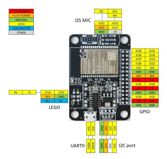
The graph above shows the pinout of the LMS ESP32 expansion board. All ESP32 GPIO pins are indicated. Where they have a specific functions, that is idicated by an extra pin label.
