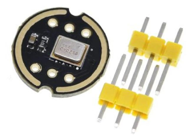
The I2S connections use GPIO 27, 32 and 33 for word clock line (I2S\_WS), the data line (I2S\_SD) and the bit clock line (I2S\_SCK). Note that this microphone is a PCM version.
