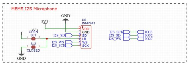
The solder pads on the back of the board can be used to select in which channel the digital output of the microphone is collected. By default the pad for selecting the left channel is shorted. Should you need to change the channel, than the trace between the MIC-L pads should be removed and the pads MIC-R should be shorted. Take care not to short both pads at the same time, as that leads to a power shortage.
