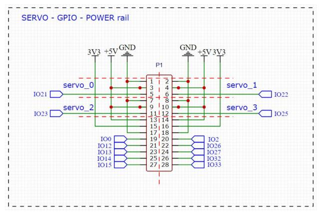
Whe grouped the pins in 3 different regions. The yellow region for connecting servo's or LED strips pwered with 5V (keep in mind that all the logic pins of the ESP32 are only 3.3V tollerant), the red region for power connections and the green region for access to the GPIO pins.
